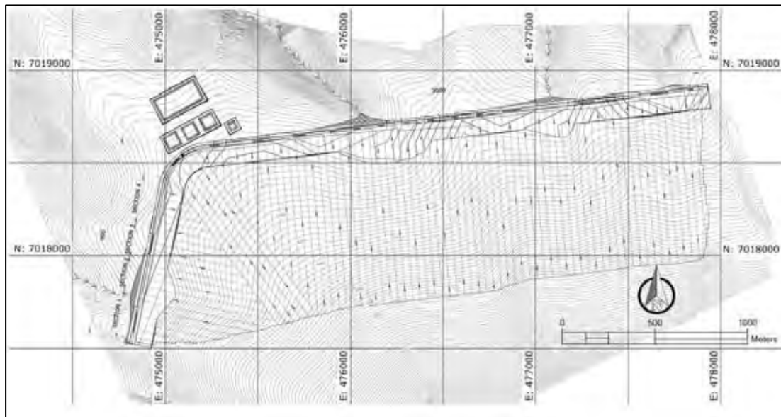
Figure 17-9 Drainage and Collection System (Plan view)
